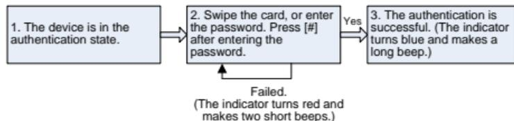
☺Note: Press [#] after entering a password for authentication. The door opens if the entered password is identical with one of the eight passwords for opening the door.
