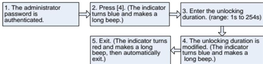
😊Note: The unit of Unlocking Duration is second. Three-digit values are automatically verified. For values with less than three digits, press [#] to enter the verification process.
