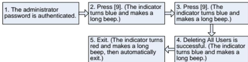
😊Note: Press [9] for automatic confirmation. Other values are considered invalid. If an invalid value is entered, the device indicator turns red, and the device makes a long beep and exits the process.
