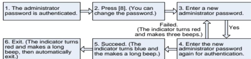
☺Note: Four-digit passwords are automatically verified. For passwords with less than four digits, press [#] to enter the verification process.
