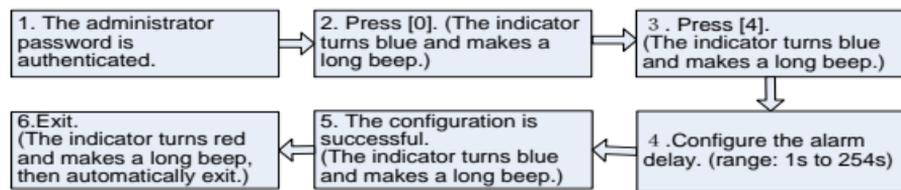
😊Note: Three-digit values are automatically verified. For values with less than three digits, press [#] to confirm. Values greater than 254 are considered invalid.
