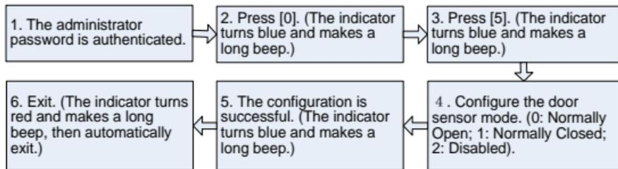
☺Note: The door sensor mode configured here is used as the basis for the door sensor alarm.
