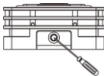
Remove the screw on the bottom of device.
