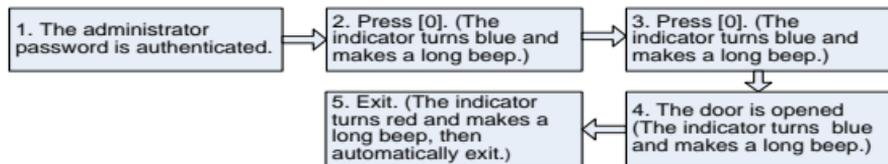
😊Note: This function can be used to open the door.
