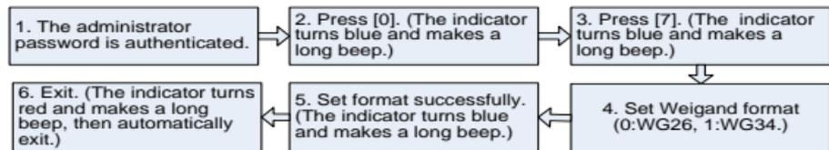
☺Note: The device makes three short beeps when fails in setting, then the indicator turns red and makes a long beep, then automatically exit.
