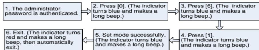
😊Note: The device makes three short beeps when fails in setting, then the indicator turns red and makes a long beep, then automatically exit.
