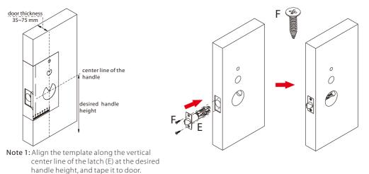
Note 2: Mark the holes first, then start drilling.
