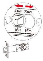
Note1: Installation template has the backset options of both 60 mm and 70 mm.
