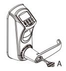
Step1: Insert the equipped tool into the hole. Step2: Rotate the tool at 90°, then pull out the cover. Insert the key into key hole and rotate 90°.
